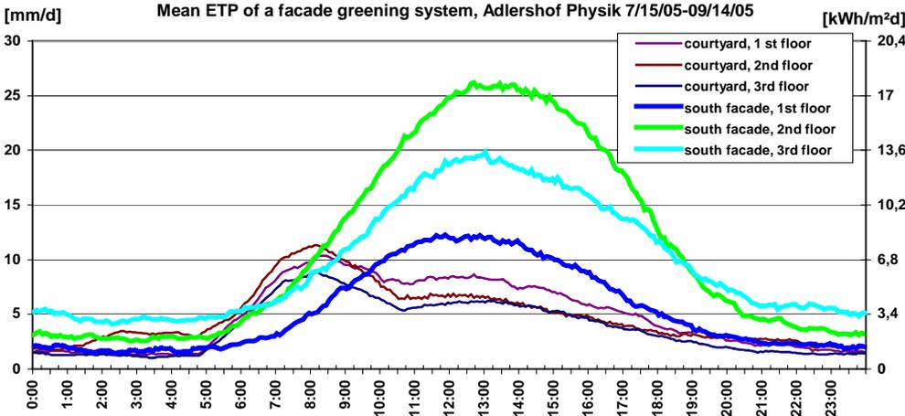
**Figure 5** mean evapotranspiration of the façade greening system in mm/day and correspondent cooling rates
