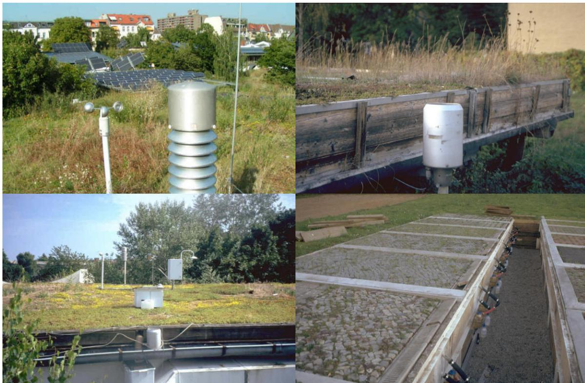
**Fig. 6-9** Measurements of precipitation and runoff at *Ufa-Fabrik* in Berlin-Tempelhof (left) and the University of Technology Berlin (green roofs and semi permeable surfaces, right)
