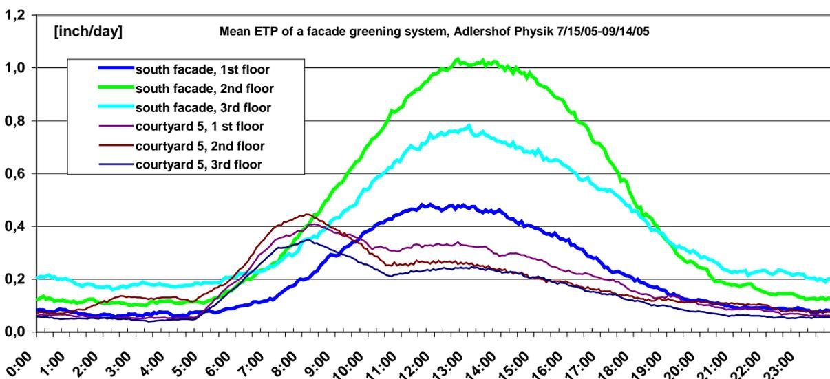
Fig. 13: Real evapotranspiration of a façade greening system, trough measurements
