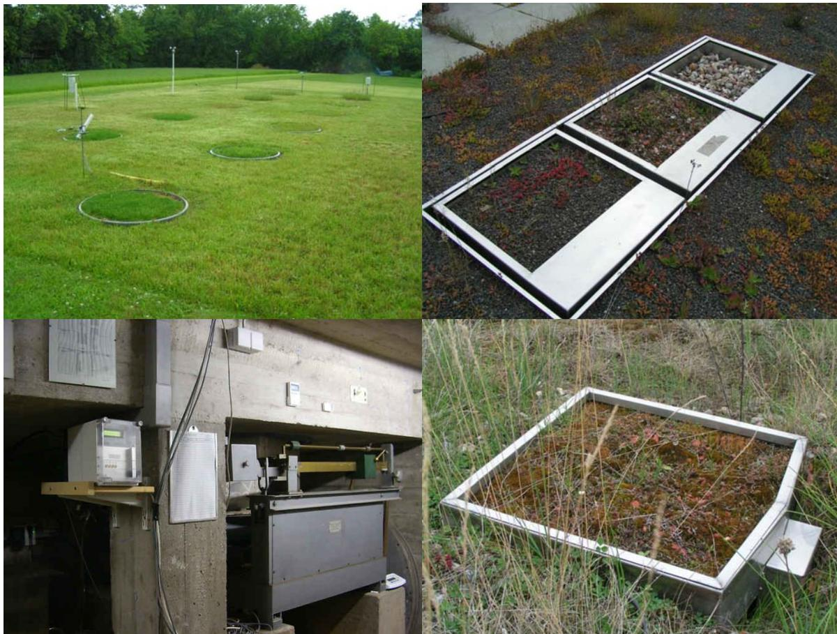
**Fig. 2-5** Lysimeter-measurements at the Univ. of Technology Berlin (soil monoliths, left, surface and underground system) and University Neubrandenburg (green roofs, right)
