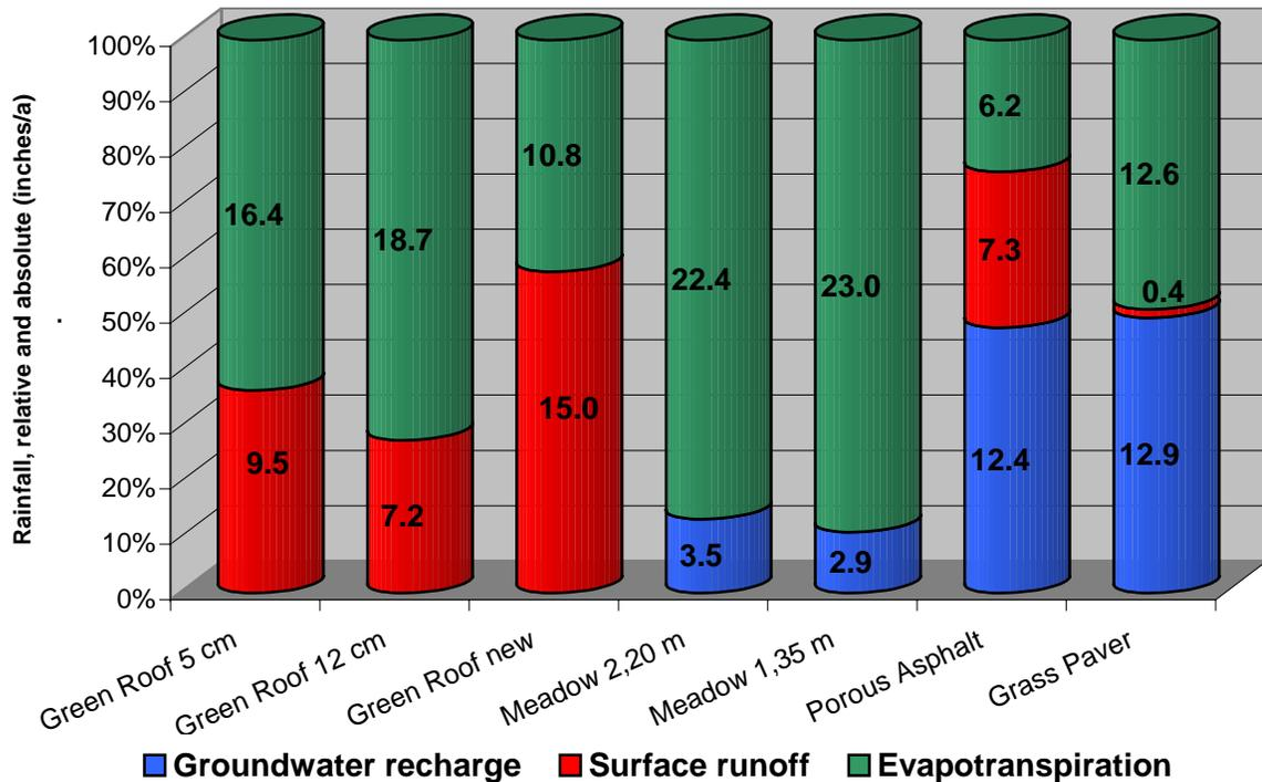
**Fig. 1 Hydrology of different surfaces (inches/a and %), 1/1/2001 – 12/31/2004
