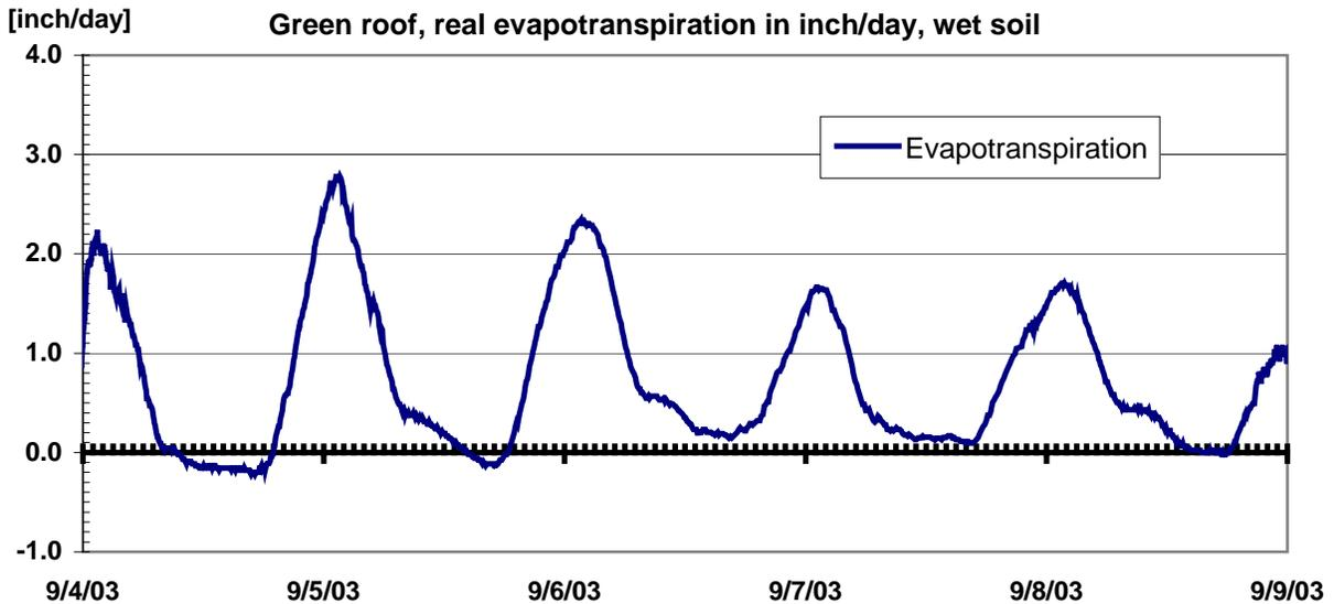
**Fig 12: Real evapotranspiration of a greened roof, lysimeter measurements**
